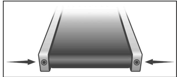
DO NOT OVER TIGHTEN – Over tightening will cause belt damage and premature bearing failure. If you tighten the belt a lot and it still slips, the problem could actually be the drive belt—located under the motor cover—that connects the motor to the front roller. If that belt is loose it feels similar to the walking belt being loose. Tightening the motor belt should be done by a trained service person.
